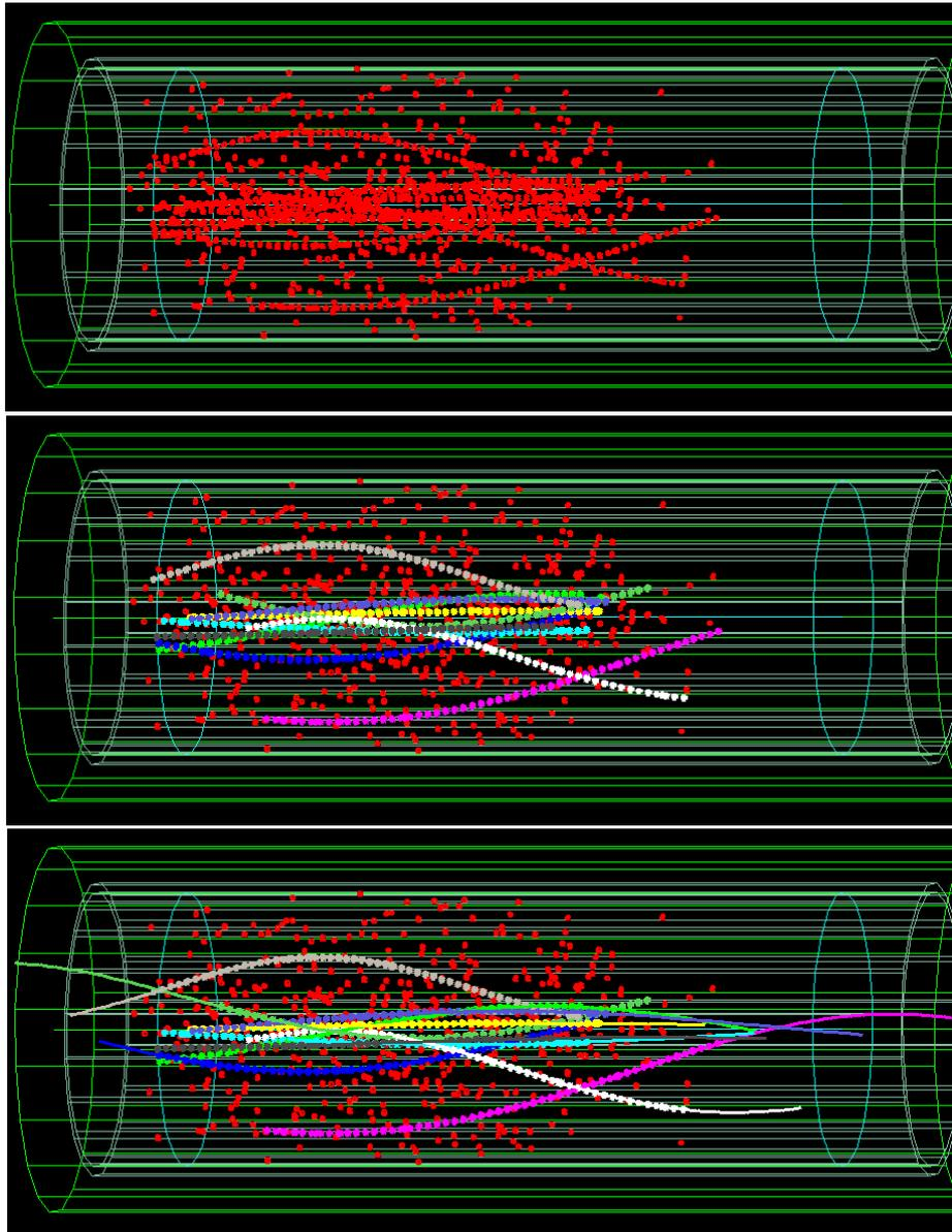
**Figure 13:** top: simulated track and noise hits in the TPG; middle: highlighted hits are those assigned by the pattern recognition to belong to the same track; bottom: track fitted on the selected hits.
