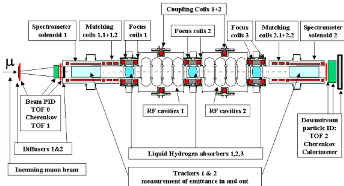
**Figure 10 :** layout of MICE, the International muon ionization cooling experiment.
