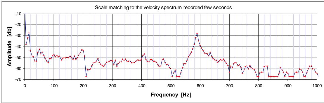
**Figure 6 :** Measurements of the horn vibration frequencies using a laser vibrometer.
