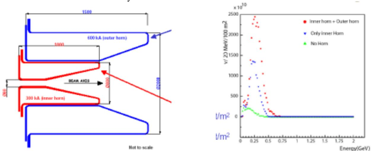
**Figure 7 :** Double horn concept and improvement in the flux for the low energy superbeam.
