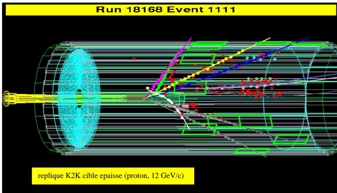
**Figure 8** : 3D view of a 12 GeV/c proton interaction in the HARP TPC, showing the raw TPC hits and the reconstructed tracks.
