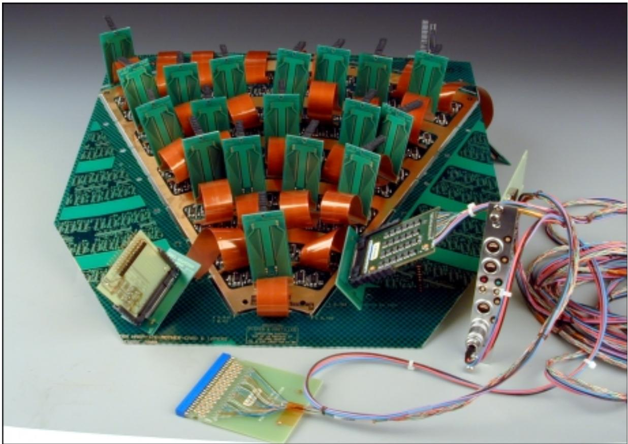
**Figure 9:** One of the motherboards of the TPC readout sector chambers, showing the "micro-flex" cables.
