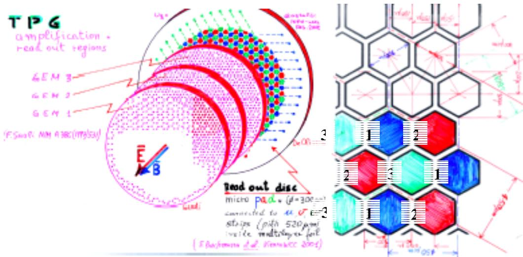
**Figure 12** : TPG readout: left: the 3 GEM foils provide amplification onto the hexaboards. Right: the hexaboards with one third of the pads (blue) connected in strips at 30°, one third at 150°
