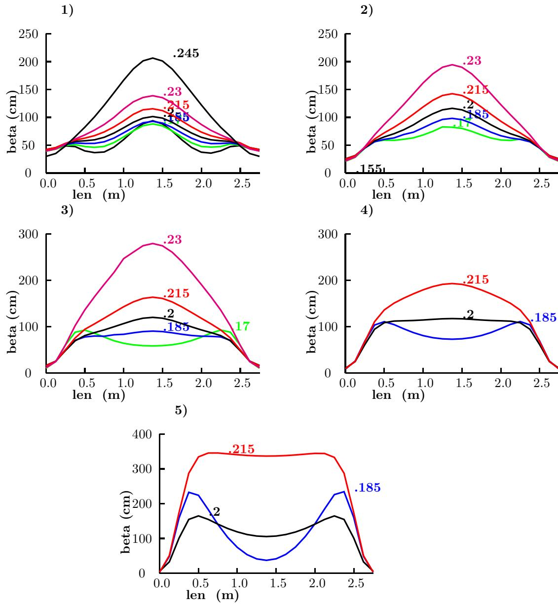
The maximum beta functions for the lowest beta minimum cases are a little higher. But this does not mean that larger apertures are required because the low minimum betas would be used only for low emittance beams.
