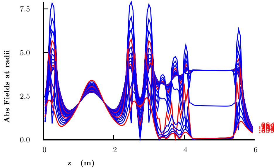
From this plot we can obtain approximate maximum fields seen by the conductors. These fields, together with the other coil specifications are given below:
