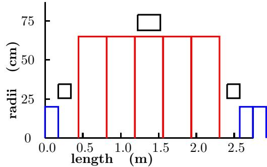
With the same coil dimensions, changing the currents can change the minimum  $\beta_{\perp}$ 's. In the following table the current densities, for a beam momentum of 200 MeV/c, are given for 5 different cases:
