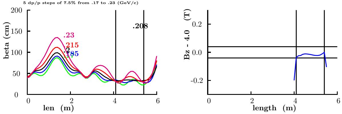
It is seen that this case is not achromatically matched: momenta other than the central one oscillate in the detector solenoid. A measure of the quality of the match is  $\delta$ : the sum in quadrature of the maximum relative beta errors:
